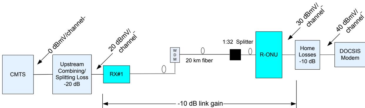
**Figure 8: Example of FM system link gain**
