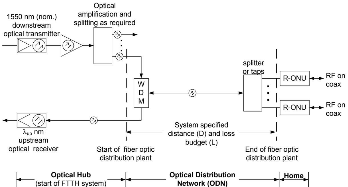
**Figure 2: RFoG Reference Architecture**
