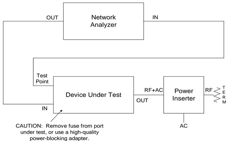
**Figure 2 – Input Port Test Point Measurement**
