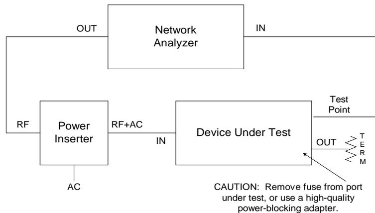
**Figure 4 – Output Port Test Point Measurement**
