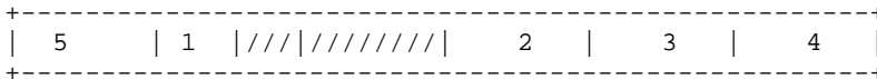
Figure 6.5. The order from 1 to 5 in which the sub-blocks are encoded. The slashed area is the start state.
