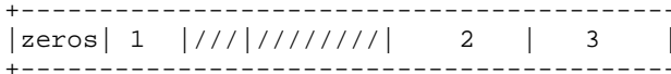
Figure 6.8. The codebook memory, length lMem=147 samples, and the target vector 3, length 40 samples
