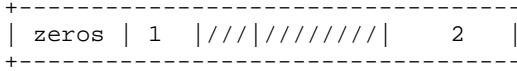
Figure 6.7. The codebook memory, length lMem=147 samples, and the target vector 2, length 40 samples
