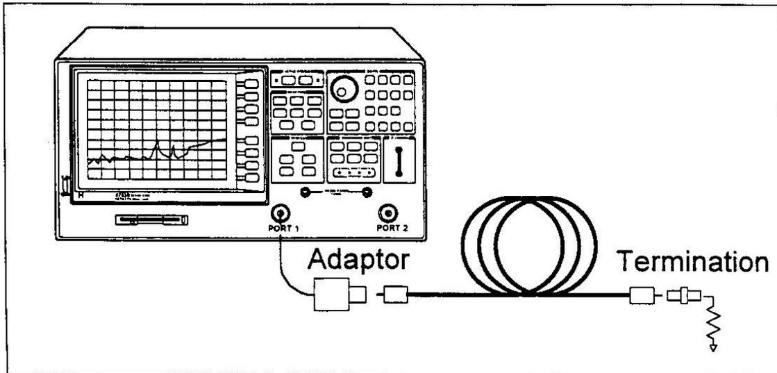
Figure 3: Instrument Setup for Fixed Bridge Method
