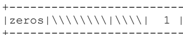
Figure 6.6. The codebook memory, length IMem=85 samples, and the target vector 1, length 22 samples
