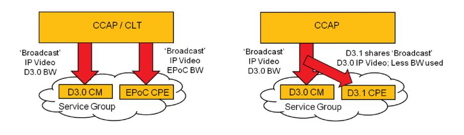
This example: EPoC requires IP Simulcast Overhead; D3.1 has none
