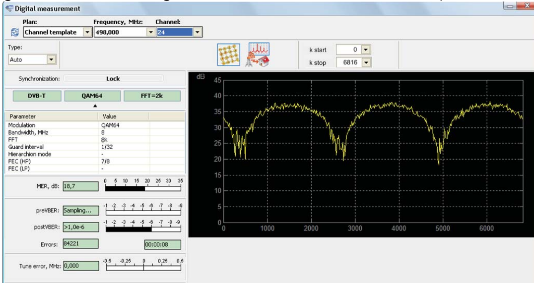
Figure 3 – OFDM test receivers can display MER versus subcarrier in graphical format. Here the MER of a 64QAM DVB-T channel is shown for subcarriers 0-6816. MER ranges from 37 dB to less than 25 dB, perhaps due to a strong micro-reflection in the network.
