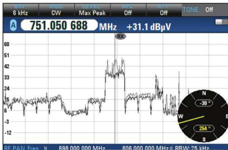
Figure 5. Leaking QAM signals in the 698-806 MHz LTE band
