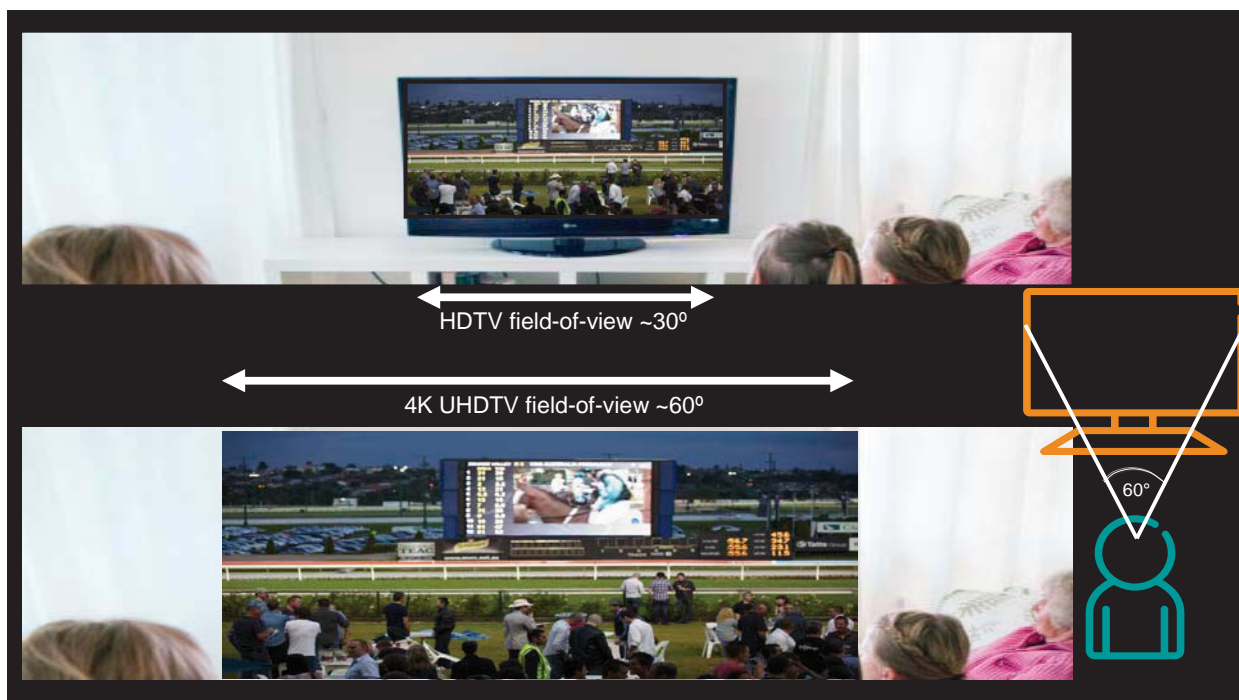
Figure 2. Comparison of 4K UHD TV and HDTV field of view within human central field-of-vision (approximately 90 degrees).
