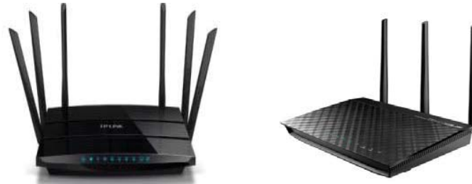
Figure 22: MIMO Using External Antennas
