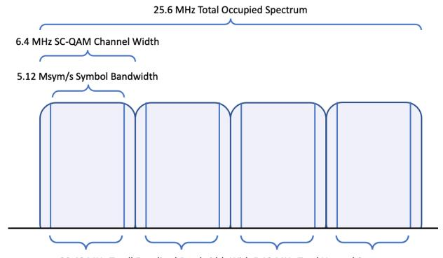
20.48 MHz Totall Equalized Bandwidth With 5.12 MHz Total Unused Spectrum
