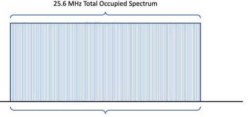
25.6 MHz Totall Equalized Bandwidth at 50-kHz Subcarrier Spacing
