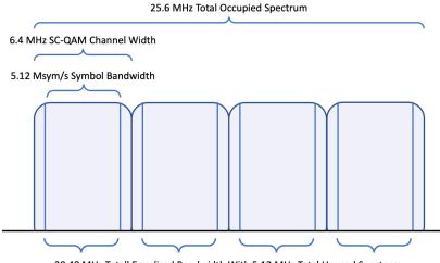
20.48 MHz Totall Equalized Bandwidth With 5.12 MHz Total Unused Spectrum
