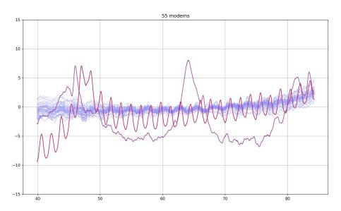
Figure 5 – Two modems under impairment with different signatures
