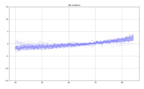
Figure 4 – Multiple modems' pre-equalizer amplitudes on a node
