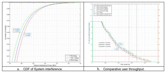
Figure 4 Vtilt impact upon system interference and the related user throughput degradation as a function of Elevation Vtilt=0°/-15°/-21° ( $h_{BS}$ =60m, outdoor scenario, NetLoad=50%, <u>95%</u> Service Availability, 3.7GHz).
