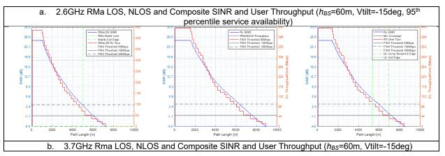
Figure 11. Comparative LOS, NLOS and Composite SINR and Tput, 2.6 3.7GHz<sup>2</sup>
