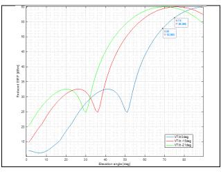
Figure 3. BS Antenna Tilt Impact upon EIRP Distribution vs. Elevation Angle (Reference Boresight Horizontal Direction), 3.7GHz (*h<sub>BS</sub>*=60m).
