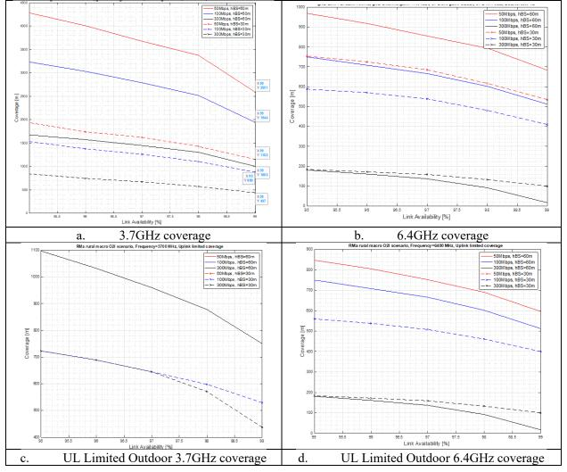
Figure 13. Comparative O2I (*h<sub>BS</sub>*=30 and 60m) Coverage, for 3.7 and 6.4GHz, When Subject to UL Coverage Limitations
