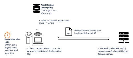
Figure 2 - Intelligent Buffering over the 10G Network
