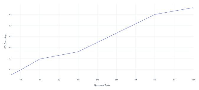
Figure 10 – ng-CCF's CPU usage (16-core) with different numbers of tasks
