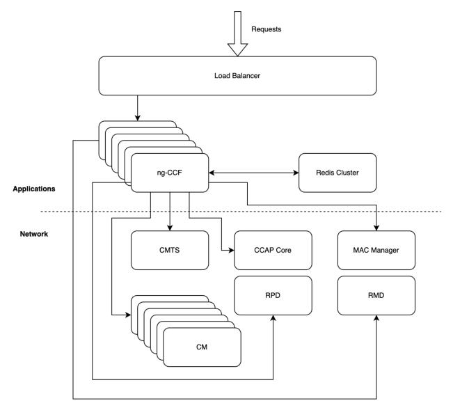
Figure 6 – ng-CCF deployment architecture (horizontal scaling)
