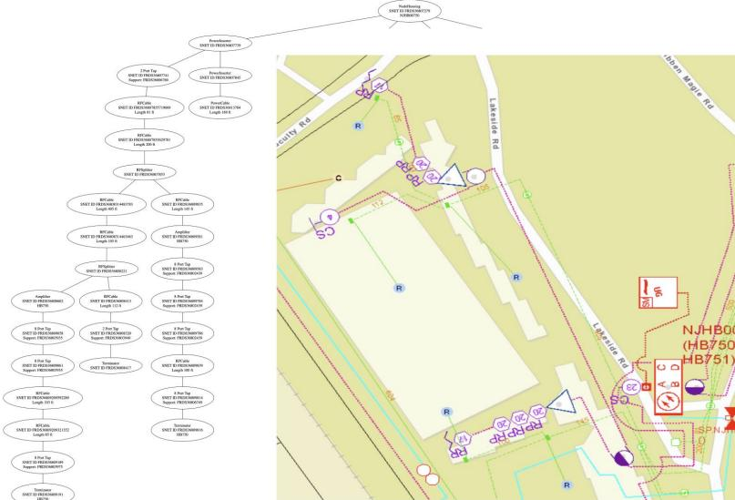
Each RF cable or RF equipment element is represented by a vertex in the graph. Edges in the graph represent connectivity.
