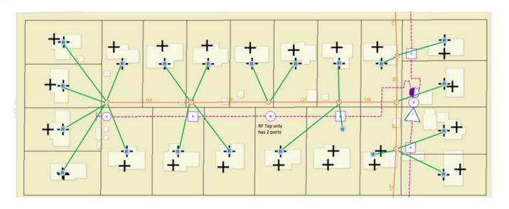
Addresses must be associated to RF taps in the graph to find map inconsistencies, calculate homes passed and device counts, and find the node segment per bus leg.
