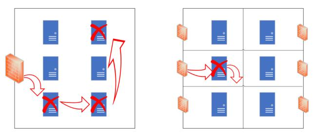
Figure 7 – An Unsegmented Network and a Microsegmented Network
