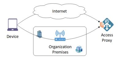
Figure 10 – Converged Access Proxy Architecture
