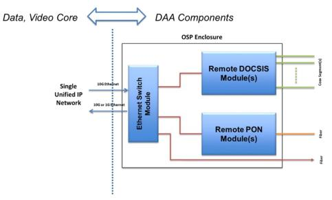
Figure 5 – DAA Enables Access-Agnostic IP Network Architecture Convergence
