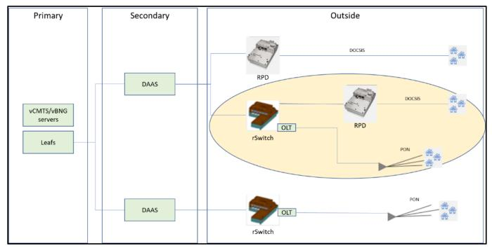
Figure 2 – DAA Basic Infrastructure Demonstrating Converged Access
