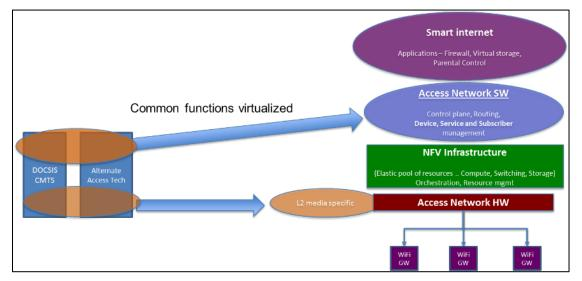
Figure 3 – Virtualization of Edge Access Platforms
