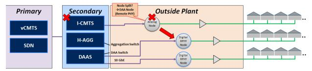
Figure 4 – Comcast DAA Architecture based on Remote PHY Node and vCMTS
