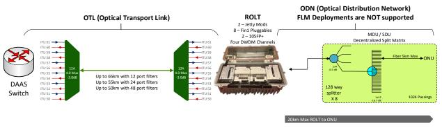
Figure 11 – DAA-Based PON – Optical Connectivity
