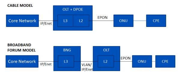
Figure 6 – Cable and Telco PON Network Models
