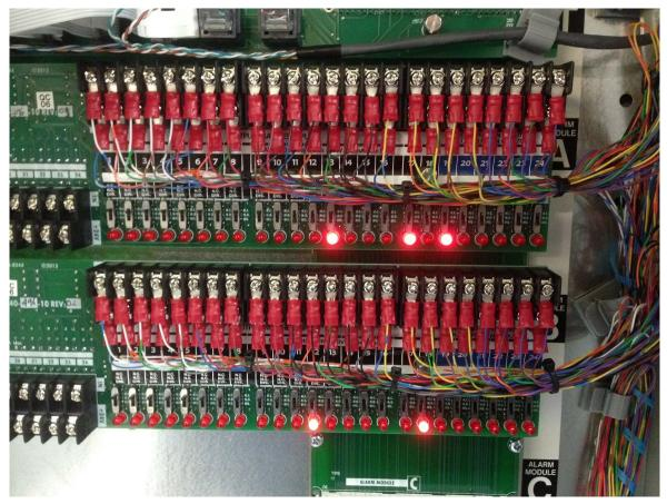
Figure 4 - Traditional Dry Contact Telemetry
