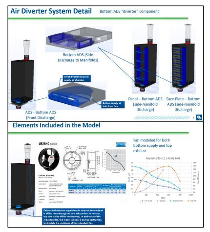
Figure 6 - Air Diverter System (Courtesy of Chillirack)
