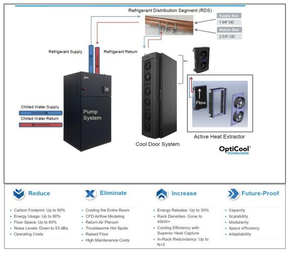
Figure 5 - Rear Door Cooling ( Diagram credit: OptiCool )
