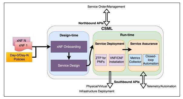
Figure 4 - High-level CSML architecture
