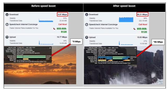
Figure 8 - Speed test results and 4K video connection speeds before and after speed boost
