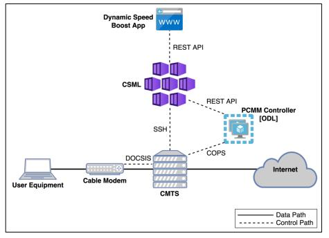
Figure 6 - Network topology of dynamic cable speed boost
