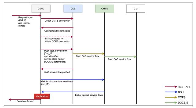
Figure 7 - End-to-end interactions of CSML with different NFs
