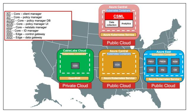
Figure 5 - Multi-cloud service orchestration using CSML
