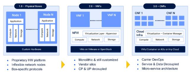
Figure 8 - Evolving from Bare Metal to VNFs to CNFs
