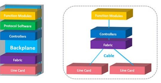
Figure 9 - DDC/DDBR Architecture
