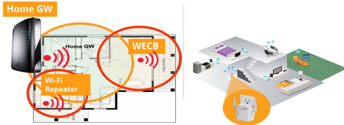
Figure 15 - Range Extension adds its own interference that needs to be managed
