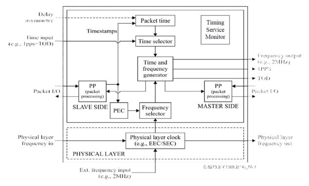
Figure 1 – Telecom Boundary Clock Model [G.8273.2]
