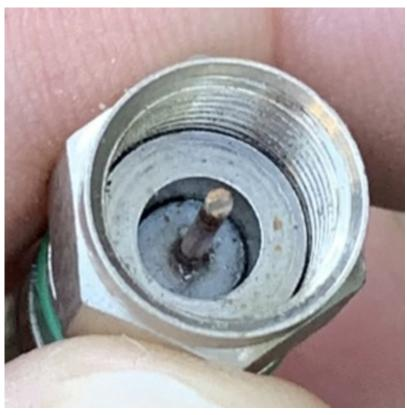
Figure 1 - F-connector not flush with the cable's dielectric
