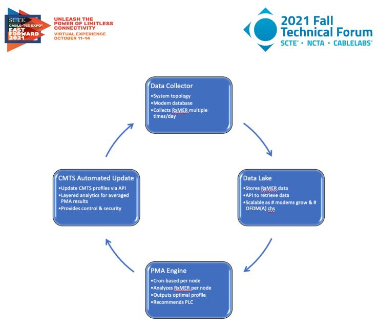
Figure 6 - PMA System Architecture.
