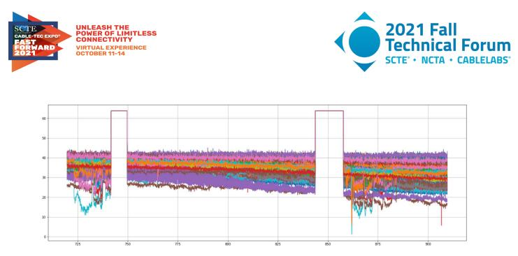
Figure 7 - Sample set from a typical fiber node with varied impairments.
