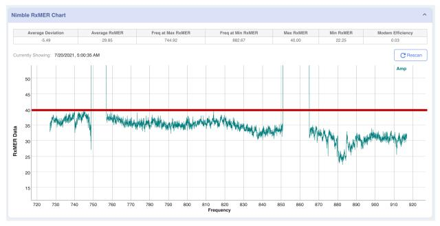
Figure 4 - RxMER per subcarrier plot of OFDM channel from live plant.
