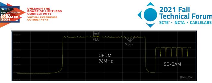
Figure 5 - Example OFDM channel highlighting the PLC [2].
