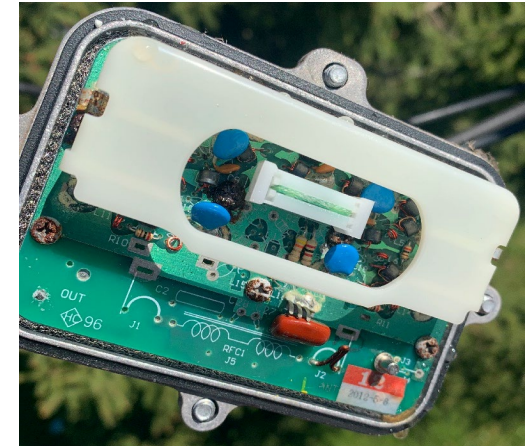
Water-soaked tap faceplate, water droplets visible
