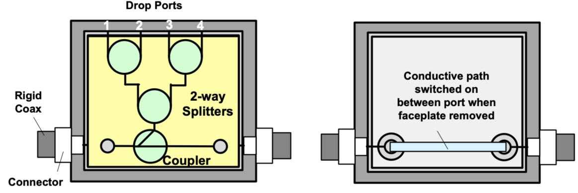
Conductive path with faceplate remove gives false sense availability as performance is degraded.
