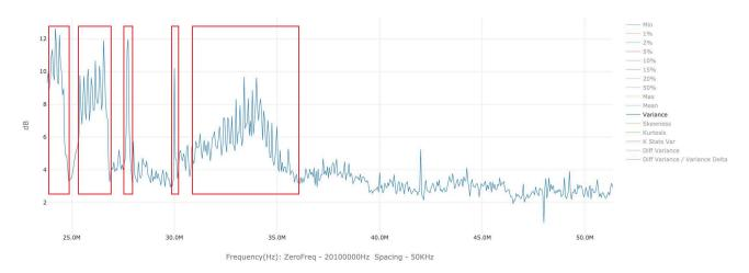
Figure 8 – Variance values calculated for each subcarrier
