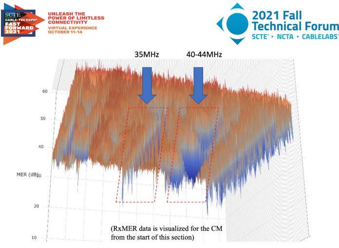
Figure 12 – 3D graph of the RxMER samples captured over time
