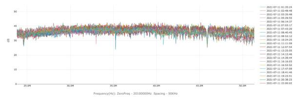
Figure 2 – Multiple US RxMER samples, OFDMA channel, Single CM (lab)
