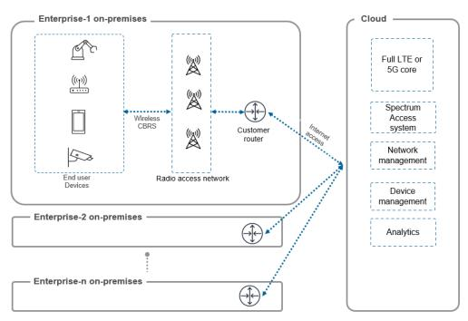
Figure 1 - Network core hosted on cloud
