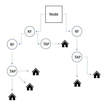
Figure 4 – Node Topology Diagram
