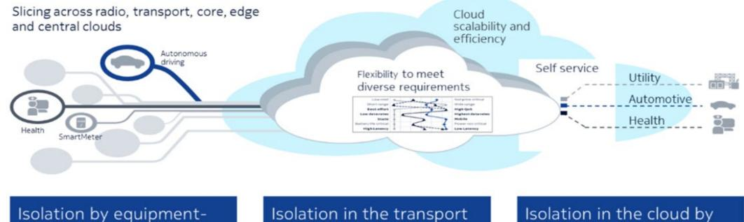
Isolation by equipmentspecific mechanisms on (non virtualized) RAN equipment Isolation in the transport by VPNs created via SDN Isolation in the cloud by NFV mechanisms in the (central/edge) cloud
