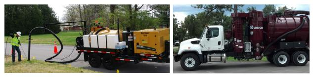
Figure 7 - Examples of Vacuum Excavators<sup>2</sup>
