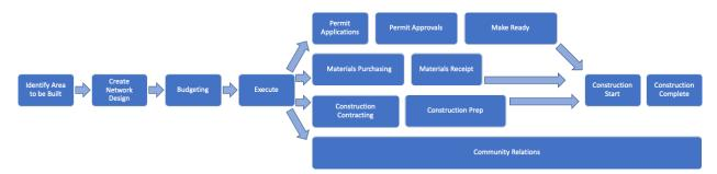
Figure 6 - Typical 1-year planning and construction cycle
