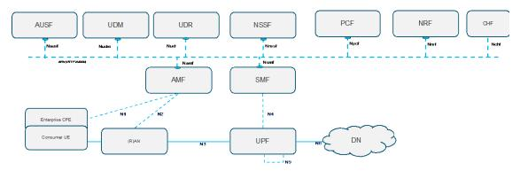
Figure 2: Simplified 5G network architecture with packet core focus
