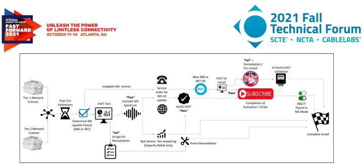
Figure 6 - Simplified Mid-Split Activation Flow: Cutover through to Activation
