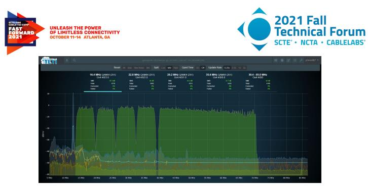
Figure 14 - High Split Yeti Screen Capture at RPD with 4 SC-QAMs and 1 OFDMA Channels
