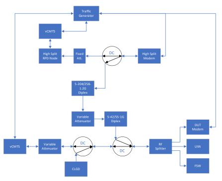
Figure 17 - Neighbor Interference for STB Test Configuration
