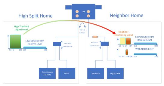
Figure 16 - Neighbor Interference in a High-Split System
