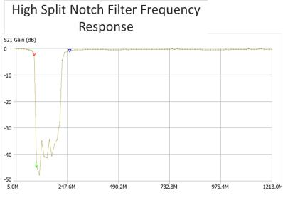
Figure 20 - Neighbor Interference Notch Filter 85-204 MHz)
