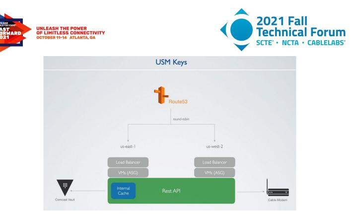
Figure 11 – SNMPv3 USM key architecture
