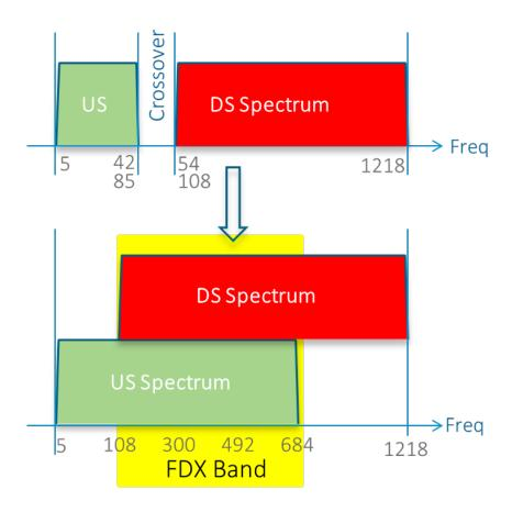
Figure 9 - FDX Spectrum Usage
