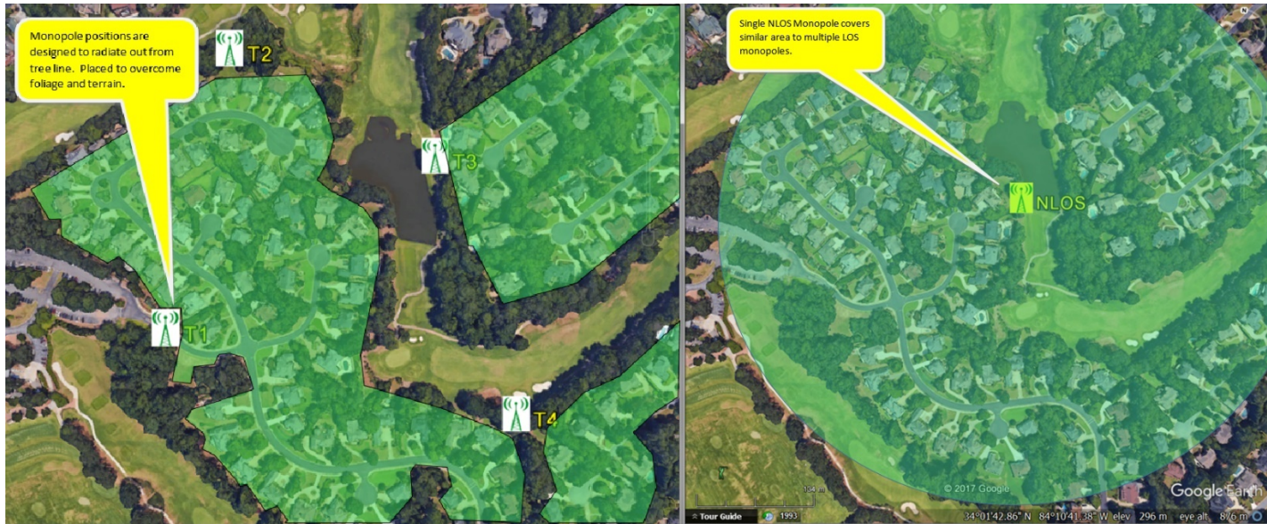
Figure 10 – Example of LOS (left) vs NLOS (right) Monopole Seeding in Golf Community Development
