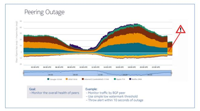
Figure 7 – ISPs can moitor peer health by setting a simple low watermark threshold.
