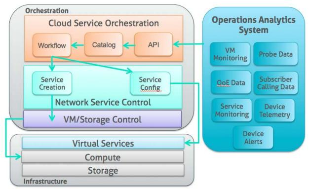
Figure 3 - Operations Analytics and Network Function Virtualization
