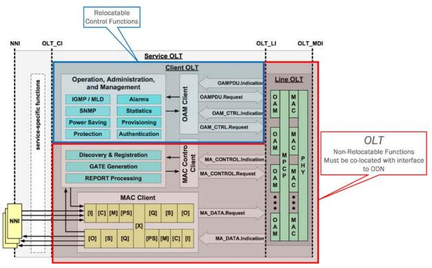
Figure 10 - Disaggregated SIEPON S-OLT
