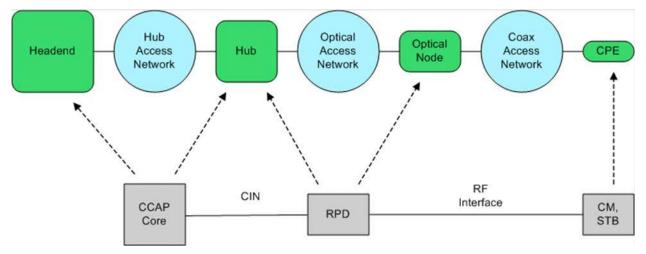
Figure 1 - Remote PHY System Diagram (Remote PHY Specification, 2017)
