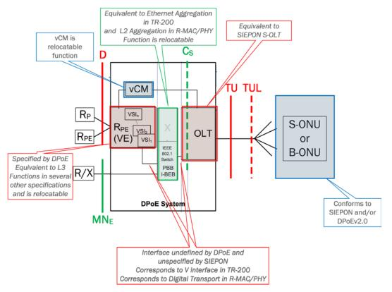
Figure 9 - Disaggregated DPoE System
