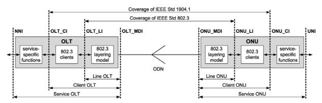
Figure 4 - SIEPON Target System Architecture with Service-Specific Functions (IEEE Standard for Service Interoperability for Ethernet Passive Optical Networks (SIEPON), 2013)
