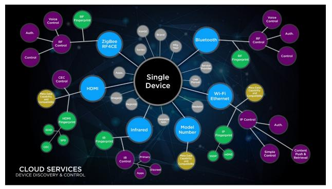
Figure 16 - Multi-Protocol Device Model with Fingerprint
