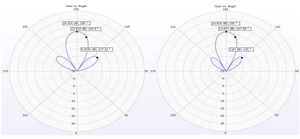
Figure 2 - 4x4 Element Array, X-Z and Y-Z Polar Plots
