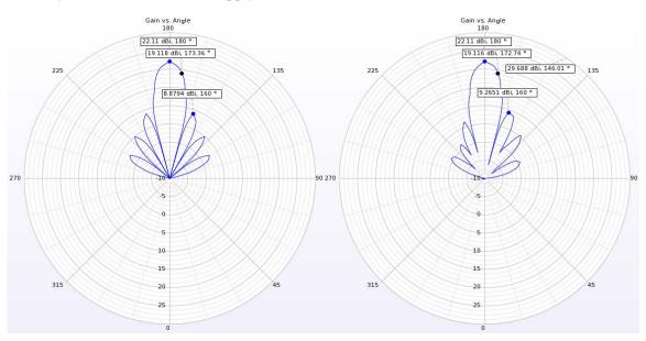
Figure 3 - 8x8 Element Array, X-Z and Y-Z Polar Plots
