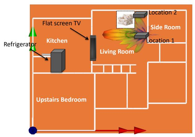
Figure 6 - Schematic of Test House Showing AP Locations
