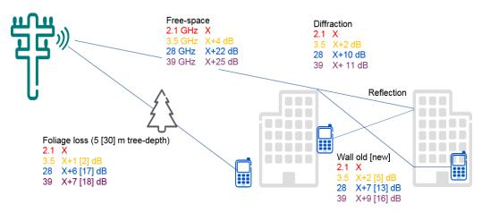
Figure 4 – Path loss comparison between spectrum bands
