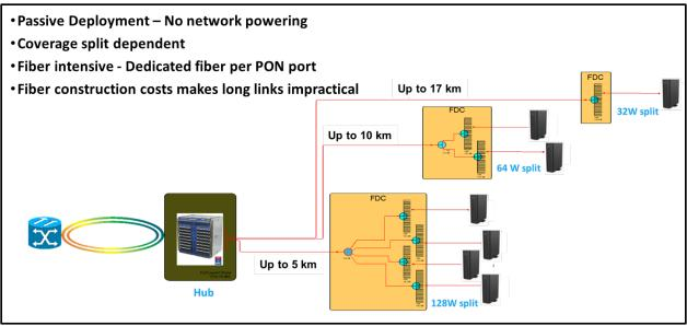
Figure 3 – FTTP Deployment Direct Feed Coverage
