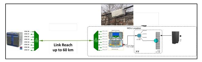
Figure 7 – 10G / 10G EPON Extender Network Configuration
