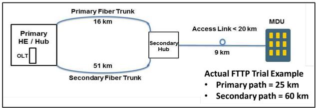
Figure 6 – Secondary Hub Limitations Can Create Extended Link Reach Situations
