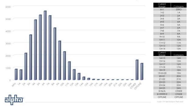
Figure 7 - Power consumption in HFC
