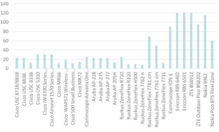
Figure 8 - Access Point Power Requirements
