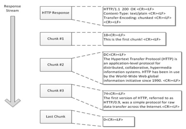
Figure 5 - Example of HTTP Chunked Transfer Encoding Response [8]
