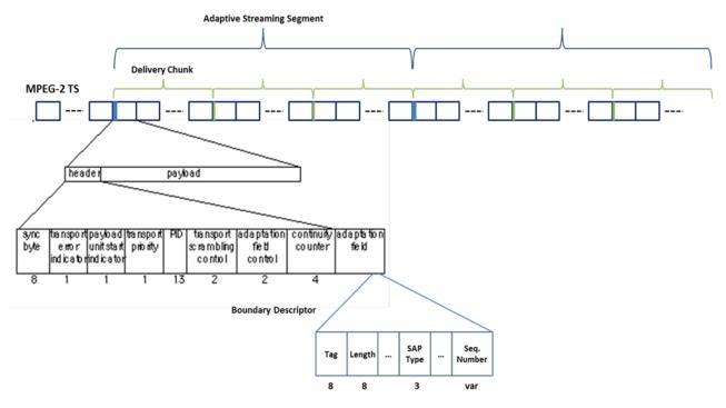
Figure 4 - Structure of Adaptive Transport Stream
