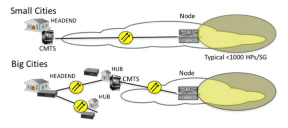
Figure 3 – Typical Cable Access Infrastructure Implementation
