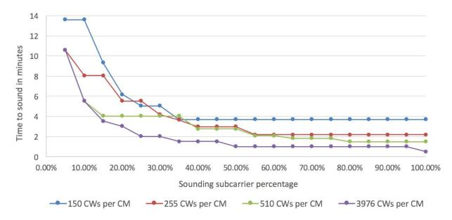
Figure 4 - CW sounding duration at different sounding subcarrier percentage and number of CWs per CM
