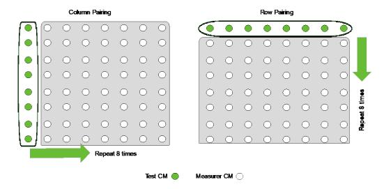
Figure 7 - Parallel sounding example
