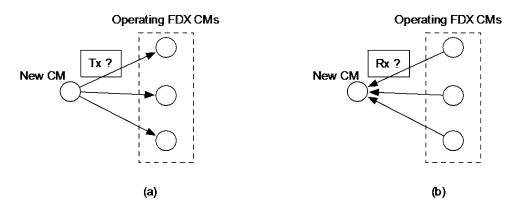
Figure 5 - Partial Sounding, (a) Transmitting Test; (b) Receiving Test
