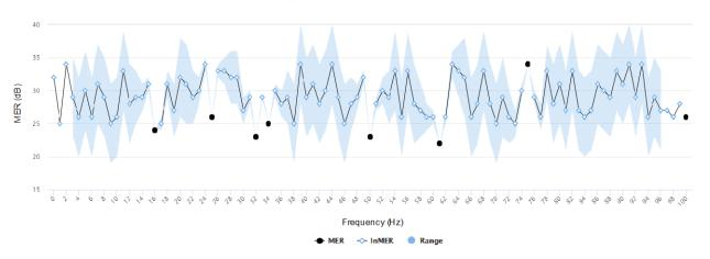
Figure 9 - Subsampling with interpolated MER (InMER) estimations
