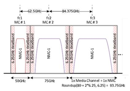
Figure 4 - Example of optical signals requiring greater than 50GHz spectrum
