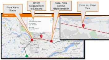
Figure 8 - Integrated OTDR Functionality
