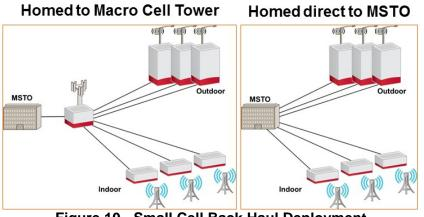
Figure 10 - Small Cell Back Haul Deployment
