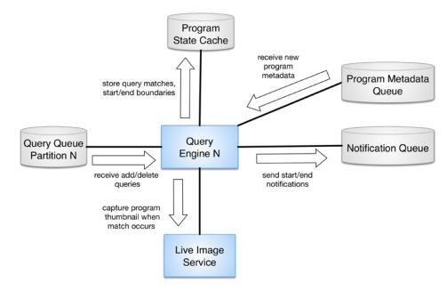
Figure 7 - Query Engine High Level Workflow
