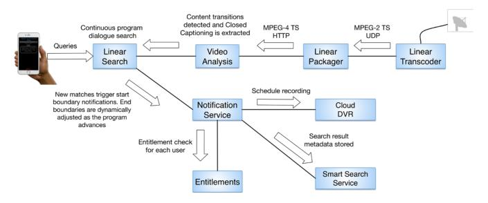
Figure 1 – Linear Search and Record Workflow Detailing System Components
