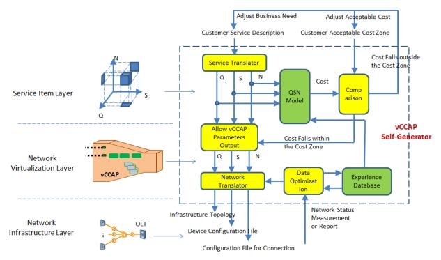
Figure 9 - Intelligent vCCAP Self-Generator Principle
