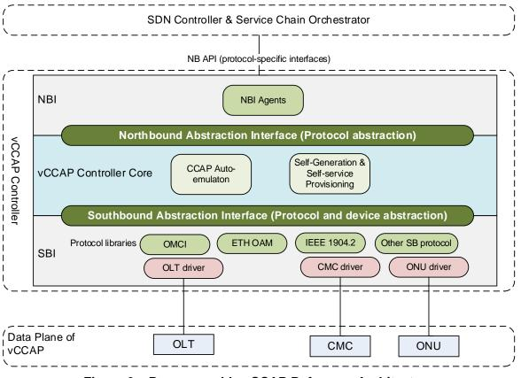
Figure 6 – Programmable vCCAP Reference Architecture
