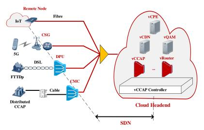
Figure 1 - High-level Architecture of Access Network Virtualization
